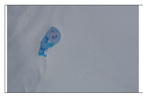
Sample nadir-looking frame camera image of a melt pond on an Alaskan icefield. Camera images are approximately 2.25 by 1.5 km at a nominal altitude of 20 km ASL.
