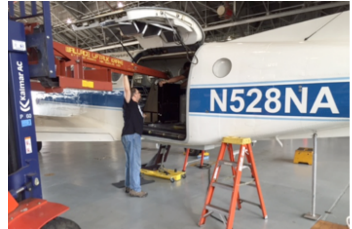
Fork lifting 150 lb SIMPL transceiver into plane
