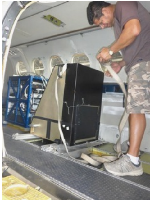
SIMPL installed over optical port behind Command and Data Handling computer rack.
