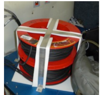
532 nm and 1064 nm fiber spools to delay TEP
