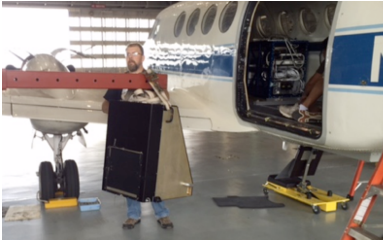
Fork lifting 150 lb SIMPL transceiver into plane
